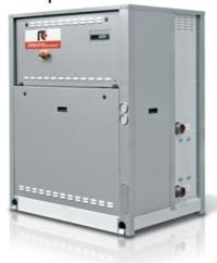
Indoor unit for the production of chilled water that may be connected to a remote condenser with hermetic rotary scroll compressors working with R410A, braze-welded plate-type exchanger and thermal expansion valve. Panels and base in hot-dip galvanised sheet steel with paint finish.
